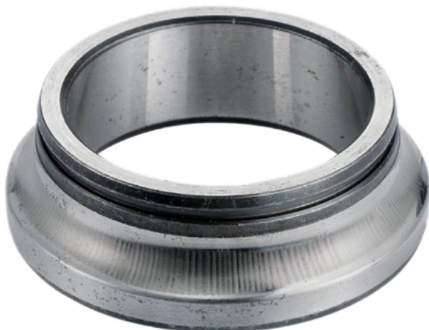
FIGURE 3 Electric erosion on a raceway [4] (© NTN)
