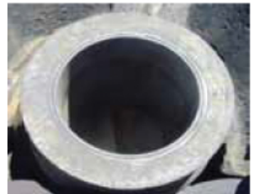
Vespel® CR-6100 3.5 year service 0.02" (0.51mm) Wear, no shaft damage Serviceable
