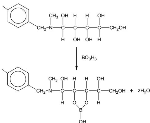
The resin has a total boron capacity of 2.6 g B/L with a capacity at 10% breakthrough of 1.5–2.0 g B/L. Once the resin is loaded with boron it can be regenerated using a mineral acid like HCl. Table 1 lists the properties of the resin; Table 2 lists recommended operating conditions.
