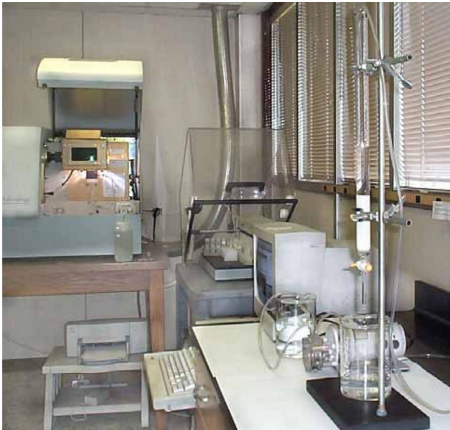
*Precious Metals Corporation conducted a laboratory experiment to determine the best ion-exchange resin for removal of boron from a process stream. DOWEX™ XUS-43594.00 resin was ultimately chosen. (Photo courtesy of Precious Metals Corporation)*
