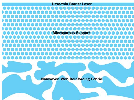
layer provides high water flux, unsurpassed salt and silica rejection, and excellent chemical resistance. The thick, microporous polysulfone support layer offers necessary porosity and strength properties and resists compaction under RO pressure conditions.
