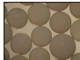
The high level of DVB crosslinker, combined with a macroporous structure, offers exceptional physical and oxidative stability, making it especially suitable for high-temperature operation. AmberLite™ HPR252 H can operate reliably under the high flowrate and pressure drop conditions that are typically used in condensate polishers.
