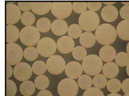
When AmberLite™ HPR8300 H is operated in the Na<sup>+</sup> form, it will remove total hardness even in high salinity waters. When operated in the H<sup>+</sup> form, it will remove only the hardness associated with alkalinity—a weak acid cation resin operated in the H<sup>+</sup> form is well-suited for use with strong acid cation resins to improve overall efficiency and throughput of a demineralization system by reducing the hardness exposure on the strong acid cation resin.
