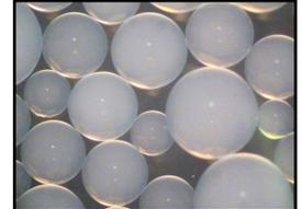
Acrylic anion resins have a hydrophilic structure providing unique chemical and physical properties allowing for easy release of the accumulated natural organic compounds during the regeneration step. The properties of the acrylic structure also enable it to withstand high osmotic or mechanical stress. The resin has been optimized to yield excellent operating capacity and efficient regeneration. Acrylic resins can be used effectively when temperatures do not consistently exceed 35°C (95°F).
