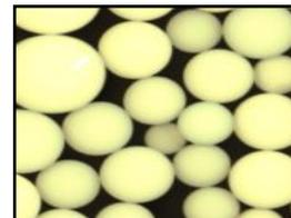
In industrial demineralization when operated in the OH<sup>-</sup> form, AmberLite™ SCAV3 Cl is ideally used as a polisher of remaining organics when placed after the anion vessel to meet the more stringent quality specifications for make-up water. Due to its strong base functionality, it will also have the ability to demineralize. When operated in the Cl<sup>-</sup> form, it can alternatively be used as a lead scavenger.
