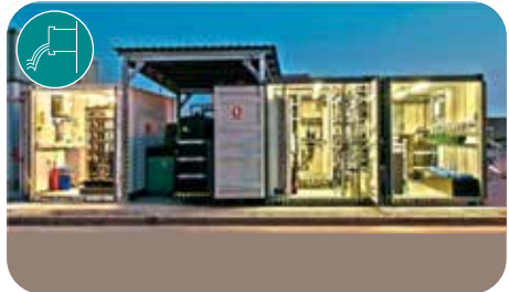
Containerized pilot plant for waste water application (UF + RO)
