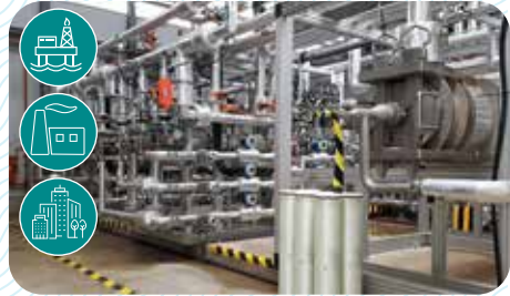
Single elements testing pilot plants (NF/RO)
