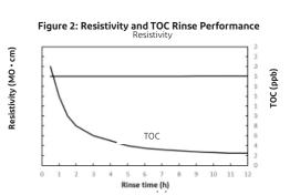
$<sup>^{\</sup>ddagger}$  Based on 18.2-MΩ• cm feedwater. AmberTec<sup>™</sup> UP6040 H/OH will deliver 18.2 MΩ• cm quality water with total organic carbon levels well below 1 ppb, in well-designed UPW systems.
