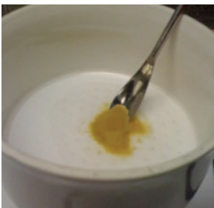
Figure 11 – Removal of Wet Cake from Filter Paper
