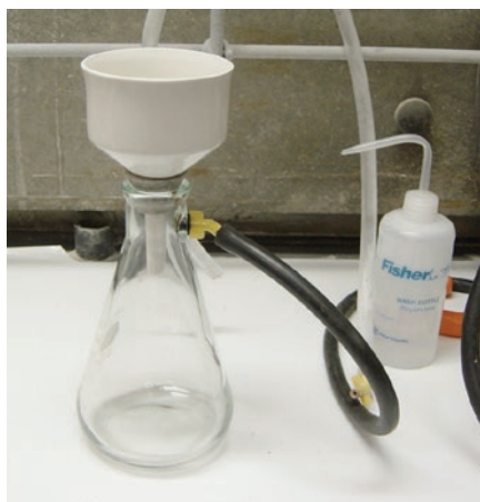
Figure 5 – Buchner Funnel Set-Up
