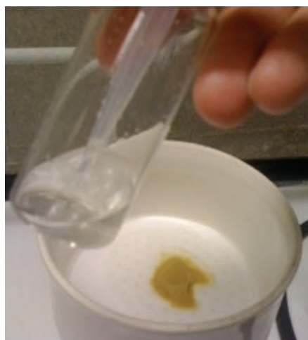
Figure 9 – Rinsing Vial and Wet Cake
