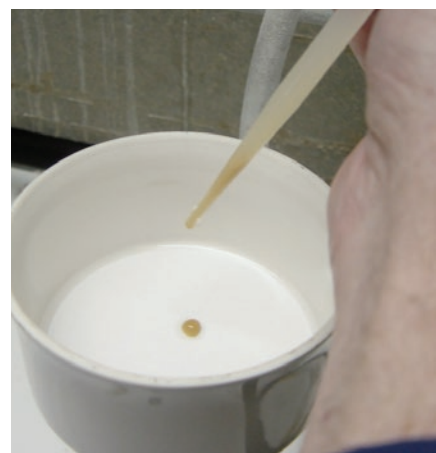
Figure 7 – Begin Transfer of Resin to Filter Paper
