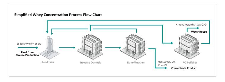
Using the on-site DWW treatment with the adoption of a multi-technology membrane combination in full-scale supports water reuse and concentration of valuable dairy ingredients, such as whey, generating additional profits for the dairy industry.
