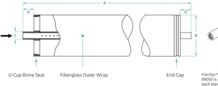
FilmTec™ coupler part number 89055 is ordered separately for each element. Each coupler includes two 2-210 EPR O-rings (part number 89255).
