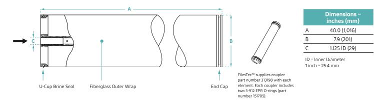
1. For element weight information refer to <u>What is the weight of FilmTec™ elements as delivered?</u> (Form No. 45-D04811-en)
