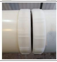
d) Hold the module and attach the second spacer ring over the protruding end of the module
