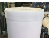
c) Put the 2<sup>nd</sup> module on the DuPont<sup>™</sup> interconnector of the 1<sup>st</sup> module and push the package carefully into the pressure vessel (30-50 cm should remain outside)
