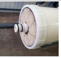
e) Insert the complete package into the pressure vessel
