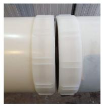
d) Hold the module and attach the second spacer ring over the protruding end of the module and insert the last DuPont interconnector into the  $4^{th}$  module
