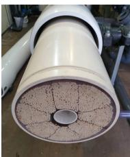
d) Hold the module and attach the second spacer ring over the protruding end of the module
