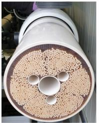
c) Hold the module and insert an  $\mathsf{DuPont}^\mathsf{TM}$  interconnector into the 1st module.
