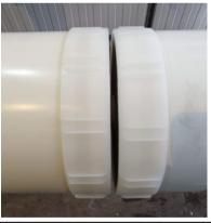
d) Hold the module and attach the second spacer ring over the protruding end of the module
