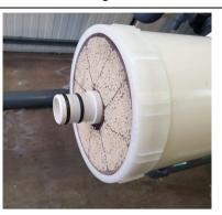
f) A spacer can be used to compensate length differences. Spacers are not part of the DuPont™ scope of supply
