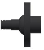
b) Shims have to be inserted on the end-cap-interconnector(s) on both sides – as needed – in order to compensate any length differences and prevent module movement during operation.
