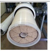
e) Insert a DuPont™ interconnector into the 3<sup>rd</sup> module
