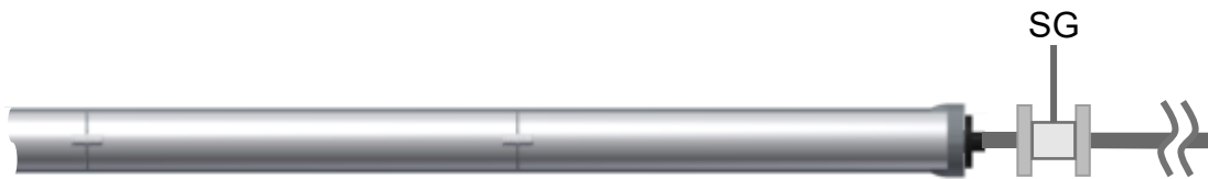
Figure 11.4-3 – Optional sight glass connected to the filtrate ports on both sides of the pressure vessels for visual observation during integrity test (bubble test) – exemplary configuration
