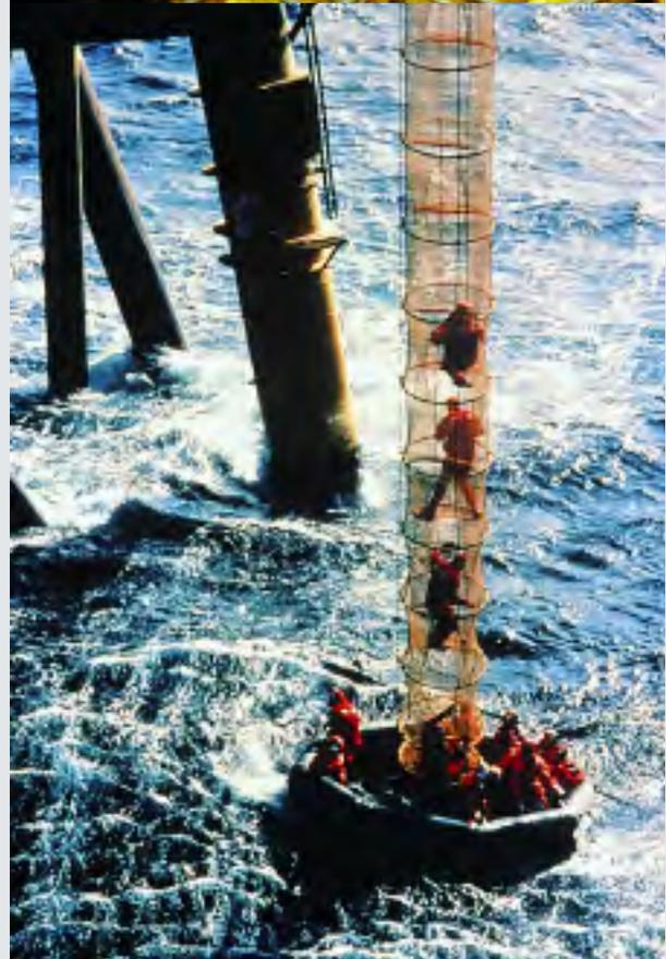
Rapid and safe evacuation of oil platforms is assured by escape chutes made of Kevlar® fibre. The chute is light, quickly deployed and corrosion, chemical and flame resistant.
