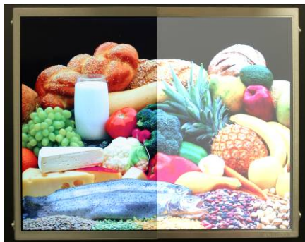
Figure 1. LCD module with bonded (L) and non-bonded (R) cover glass.
