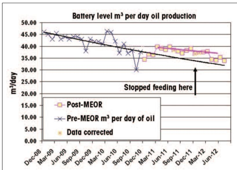
**FIGURE 2. A 15% to 20% increase in production rate was demonstrated for affected producers with a corresponding decrease in water cut after the MEOR technology was deployed.**
