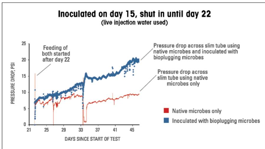
**FIGURE 1. A slim-tube pressure-drop test demonstrating bioplagging shows the contrast between using live injection water with native microbes only compared to inoculated live injection water. (Images courtesy of DuPont Sustainable Solutions)**
