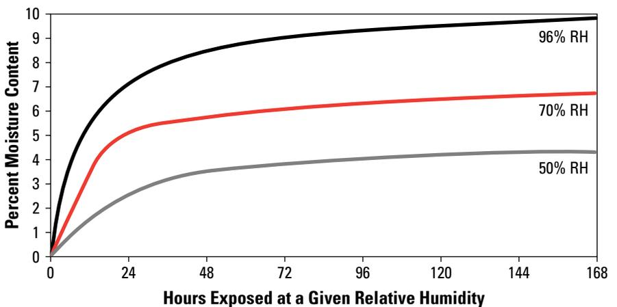
Figure 2 – MOISTURE ABSORPTION OF PRESSBOARD @ 50% RH AND 25°C
