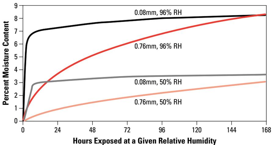
Figure 4 – MOISTURE REGAIN TIME FOR 0.25 mm (10 mil) THICK PAPER TYPES
