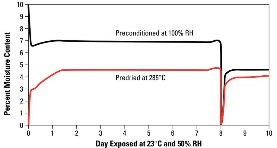
Figure 6 – **EXPANSION OF 0.25 mm (10 mil) TYPE 410 NOMEX® PAPER WITH HUMIDITY**
