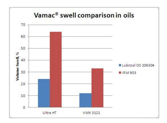
Vamac® Ultra HT-OR is the best Vamac® grade for turbo charger hoses application to pass severe oil and fluid aging requirements.
