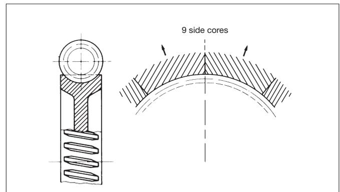
Fig. 8.14 **Side-cored worm gear**
