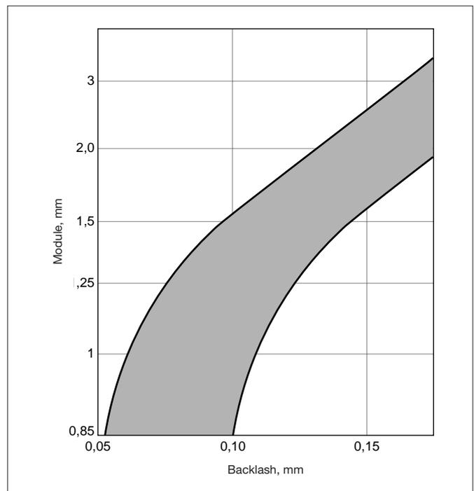
Fig. 8.12 Suggested backlash for gears of DELRIM® and ZYTEL®
