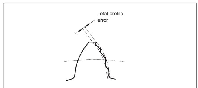
Fig. 8.11-a **Measurement of tooth profile error**
