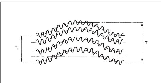
Fig. 8.11-d Moulding tolerances from center distance diagram
