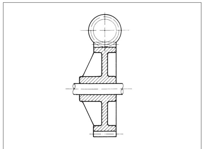
Fig. 8.07 **Ribbed worm take-off gear**
