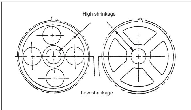
Fig. 8.08 **Holes and ribs in moulded gears**
