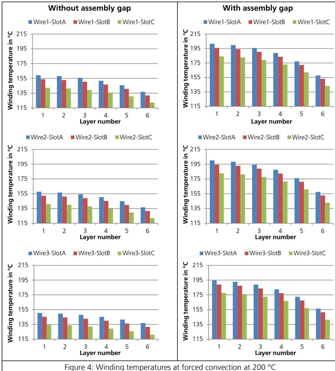
Figure 4: Winding temperatures at forced convection at 200 °C
