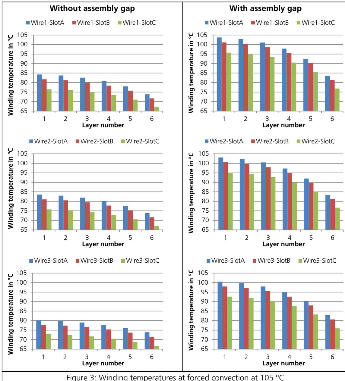
Figure 3: Winding temperatures at forced convection at 105 °C
