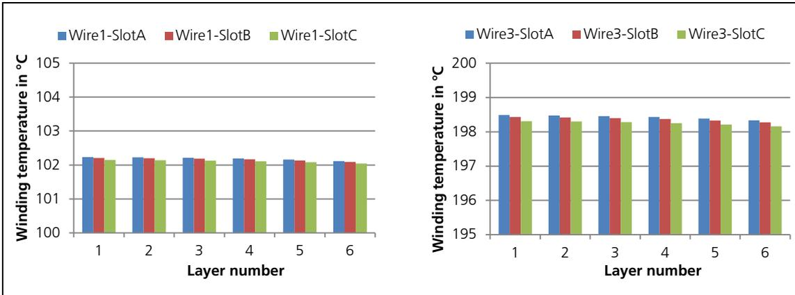
Figure 2: Winding temperatures at free convection at different end temperatures without assembly gap
