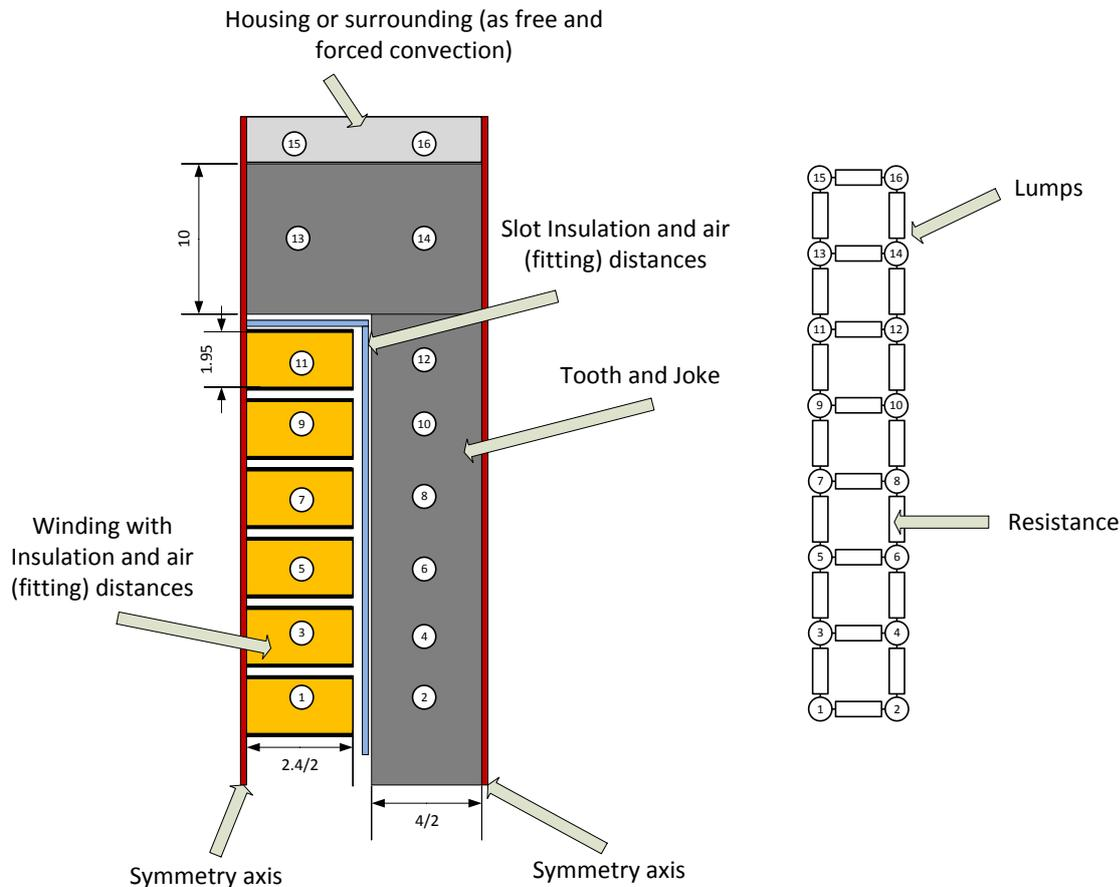
Figure 1: Lumped parameter model of a slot-tooth-symmetry unit of an electrical machine
