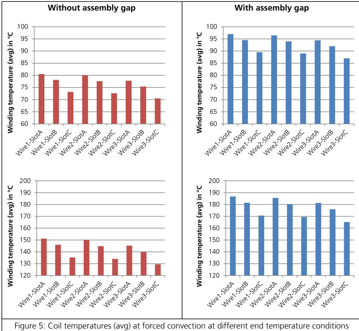
Figure 5: Coil temperatures (avg) at forced convection at different end temperature conditions
