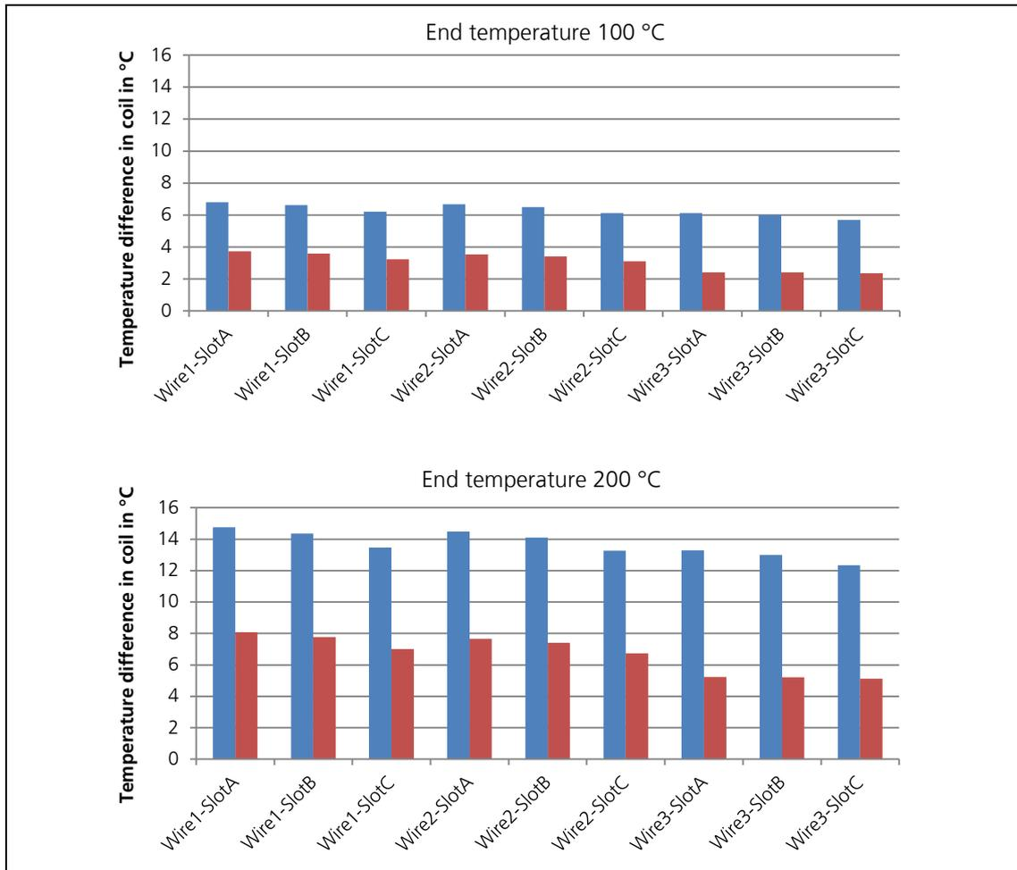
Figure 6: Temperature delta inside of the coil at forced convection at different end temperature conditions with assembly gap (blue) and without assembly gap (red)
