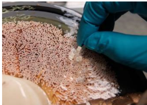
Figure 25: Identifying leaking fiber at location of large bubble
