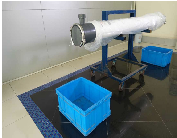
Figure 2 Liquid collection basin beneath the module ends
